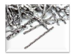
reinforcement for positive moment in floor applications in buildings. Steel fibers are used for temperature/shrinkage reinforcement in these buildings. In these applications, any concrete floor cast on a metal frame and deck system is severely restrained from movement. When the concrete shrinks, the steel frame does not. This restraint causes tensile stress to develop in the concrete, which leads to shrinkage cracks. The SDI recommends three materials to control these cracks. Which is best?
