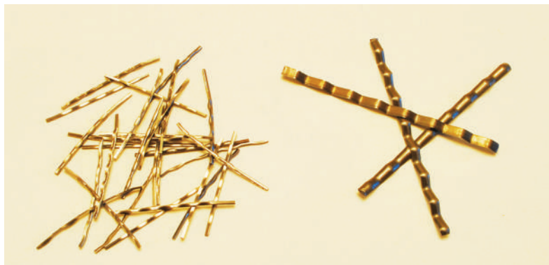
Both piles have the same mass, but the 25-mm (1-in.) fibers outnumber the 50-mm (2-in.) fibers almost eight to one.
