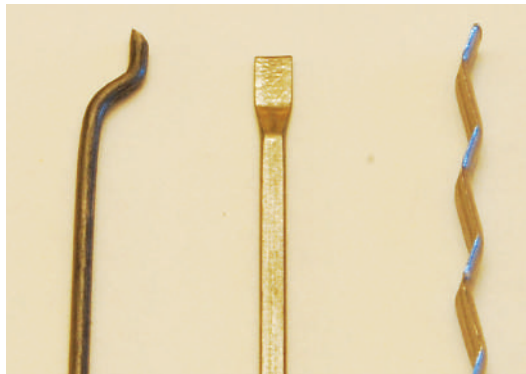
Deformations—including hooked end, flat end, and continuous—are shown here.
