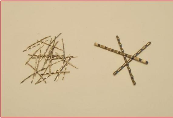
*Photo 2 - Fibers on the left are 1 inch long. Those on the right are 1-1/2 inches long. Both piles weigh the same, but the shorter fibers are more numerous and, more importantly, their total length is greater, making them better at preventing cracks.*
