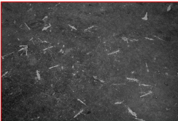
*Photo 3 - Exposed steel fibers, 2 inches long. Clearly more went wrong here than fiber length, but length was a contributing factor. Nothing as bad as this has ever been reported where 1-inch fibers were used.*
