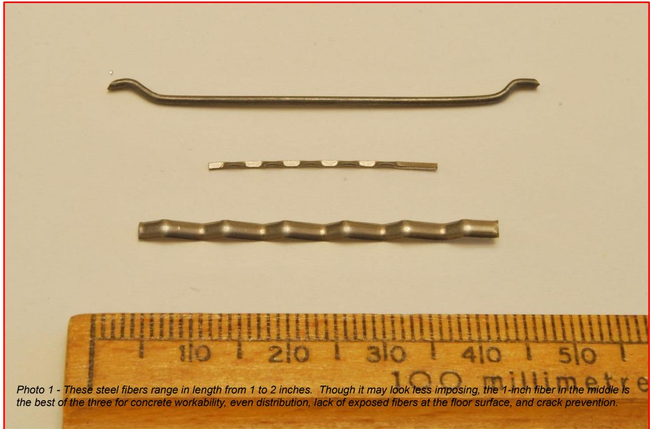
*Photo 1 - These steel fibers range in length from 1 to 2 inches. Though it may look less imposing, the 1-inch fiber in the middle is the best of the three for concrete workability, even distribution, lack of exposed fibers at the floor surface, and crack prevention.*
