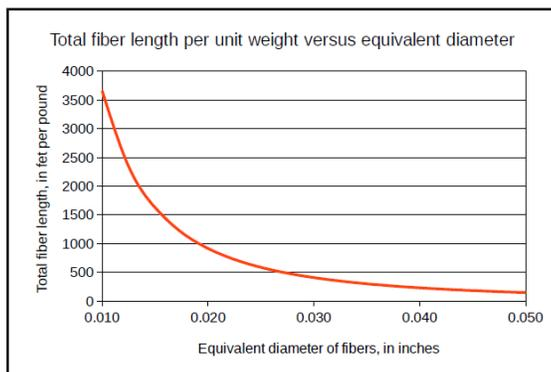
This graph shows how the total length of fibers available to intercept cracks goes up as fibers get thinner. To make fibers thin without raising the risk of tangles, you have to make them short. To move left on the graph, you need shorter fibers.
